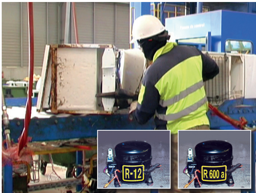
Sampling of cooling agent and cooling machine oil by means of drilling head at a compressor cooling device
