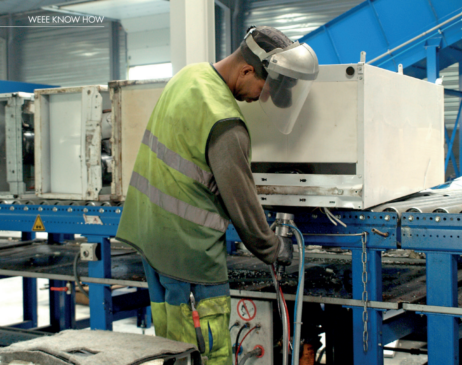
The disassembly of cooling agent compressors takes place at the end of step I plant
